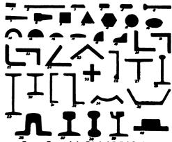
FIG. 1.-Forms of the Principal Rolled Sections.
