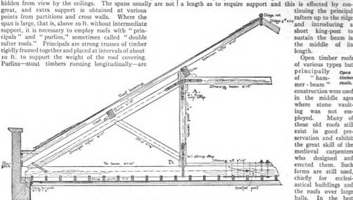
Fig. 3.-Queen-post Roof Truss; half elevation, 38' o" span
