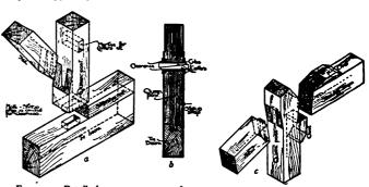
Detail of queen-post truss at b. Vertical section through queen-post. Detail of queen-post truss at head; purlin and wrought-iron straps are omitted for the sake of clearness.
