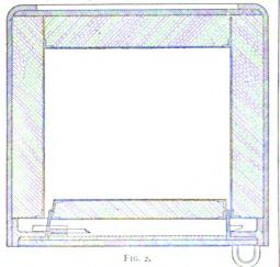
manufacture of high carbon steel, and even in what is to-day called the "fire-proof" safe a plate of steel which offers considerable resistance to drilling is placed between the outer door plate and the lock.
