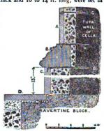
IG. 4.—Example of Marble Lining, from the Cella of the Temple of Concord. A. Slabs of Phrygian marble. B. Plinth moulding of Numidian giallo." C. Slab of cipollino (Carystian marble). D. Paving of porta santa. E and F. "nucleus" and "rudus" of concrete bedding. G, G. Iron clamps run with lead to fix marble lining. H. Bronze clamp. J. Cement backing.
