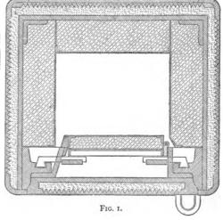
of the wrought-iron safe, as distinct from the coffer, the practice had developed of securing the door by a number of bolts operated by a handle and fastening them in the locked position by the lock proper, in order that a small key might be used (Charles Chubb's patent, 1845).
