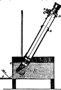
Fig. 6.-Zeiss's Dipping Refractometer.
