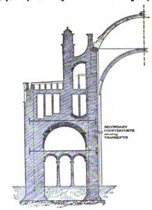
FIG. 13.-Westminster Cathedral: section through nave. on the outside. Sheets corrugated in the Italian patters have raised half-rounds every 15 in. or so, the portions between being flat. Such sheets have a very neat appearance and give a better effect in some positions than the ordinary corrugations.
