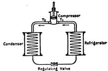
FIG. 2.-Vapour Compression Machine.
