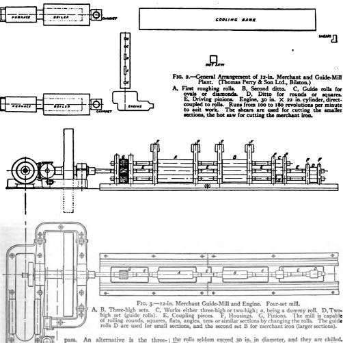
pass. An alternative is the threehigh mill, in which three rolls are used. Here the plate is run through the lower rolls and back through the upper ones, so that there is no reversal of direction of the mill as a whole, but the lower and upper rolls draw the plates in opposite directions (see also Iron and Steel, § 129).
